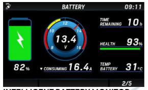
**INTELLIGENT BATTERY MONITOR screen** Dedicated screen for battery monitoring including extensive battery information coming from the Intelligent Battery Sensor (IBS).
